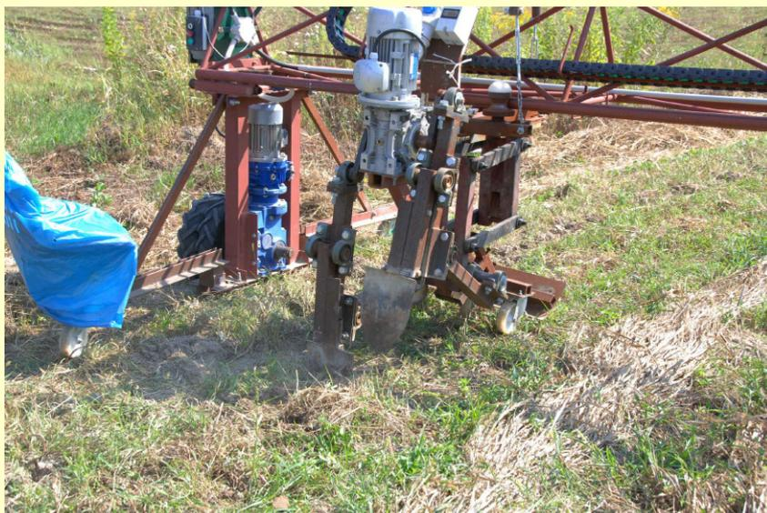
At the outer end of the Agrokruh gantry is an electrically powered drive wheel which rotates the frame around its centre. All manner of implements can be attached to the frame and these are automatically indexed inwards or outwards as the unit rotates, creating a precise spiral
